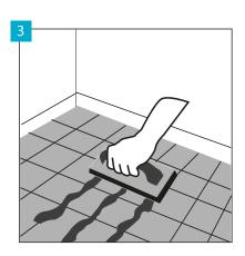
In the case of installation on the substrate covered with ceramic tiles, fill the tile joints with the gap wider than 4 mm and deeper than 1 mm with a durable compound for the filling of points, e.g. resin grout.
