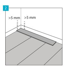
Leave 5 mm of perimeter space at the walls to allow the floor expansion.
