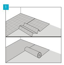
Lay the AFIRMAX underlay LVT PROTECTOR perpendicularly to the direction in which panels are laid. The neighbouring ribbons of underlay must be fit tightly and joined by means of an overlap or Arbiton AluTape, without leaving any redundant space.
