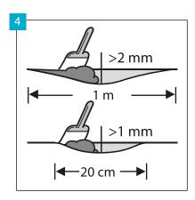
Make sure that the substrate is completely flat. All substrate irregularities exceeding 1 mm, with a length greater than 20 cm, or exceeding 2 mm with a length greater than 1 m must be levelled. Check if the use of the priming or sealing material is necessary. In order to prepare the substrate perfectly, spread the grout or the self-levelling compound on the entire surface.
