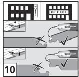
**Preparation:** Please store the packets 48 hours prior to installation under the same climatic conditions (temperature and moisture) as the actual installation process [1]. Important pre-condition for proper fitting and long-term durability of the laminated flooring is a room temperature of ca.  $20^{\circ}\text{C}/68^{\circ}\text{F}$  and a relative humidity of around 50 - 70%.
